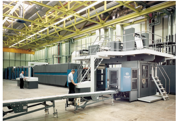
Fig. 1.2-36 Web-fed offset printing system (M-600, Heidelberg)
